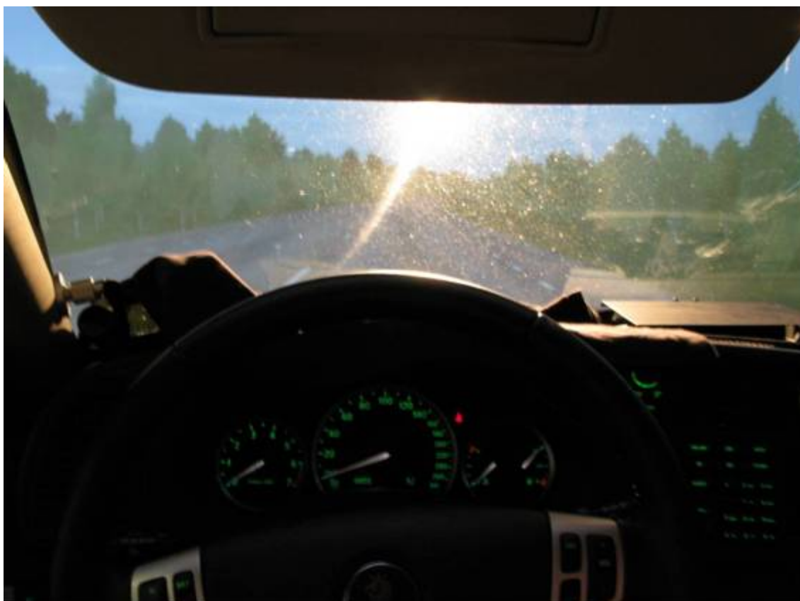
Figure 1 Driver's perspective with dazzling in the simulator. Photograph: VTI.
